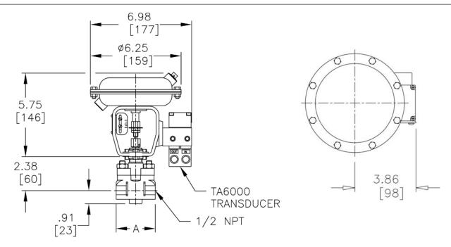
Figure 6. Dimensions - inches [millimeters] of Type 16 Actuator with TA6000 Electropneumatic Transducer (Top View on Right)
